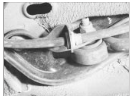
15.4 Tie-bar bracket on the underbody
