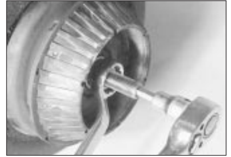
5.4 Unscrewing the nut from the top of the strut
