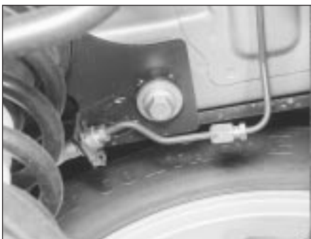
26.7A Rear suspension crossmember rear mounting bolt
