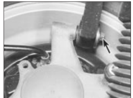
24.3 Bolt (arrowed) securing the upper arm to the knuckle
