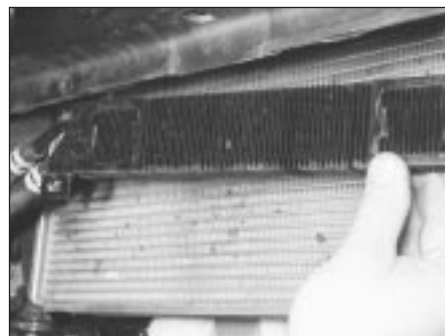
1.5 The power steering system fluid cooler is located in front of the radiator
