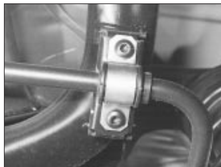
20.3 Anti-roll bar mounting clamp on the rear suspension crossmember
