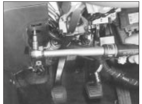
28.13 Tightening the steering column mounting bolts
