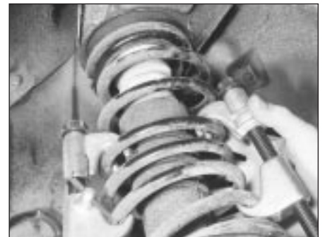
11.14 Removing the rear suspension strut
