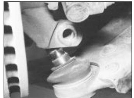
7.7B . . . and disconnect the balljoint from the knuckle
