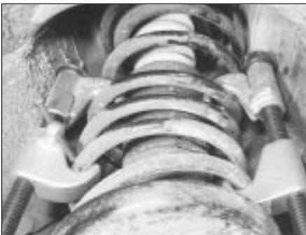
11.12 Compressor tools fitted to the rear coil spring
