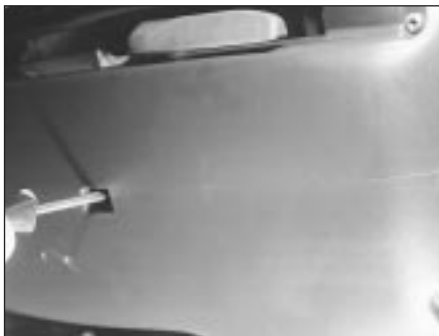
28.4A Unscrew the screws from the lower shroud . . .
