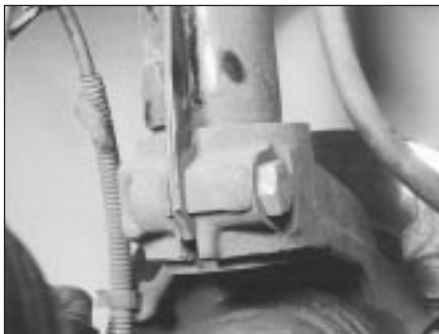
4.12A Steering knuckle-to-strut pinch-bolt
