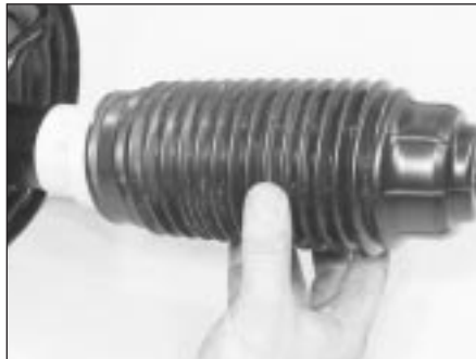
5.5C Removing the gaiter
