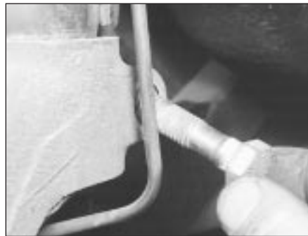
11.10B . . . and remove the knuckle-to-strut clamp bolt
