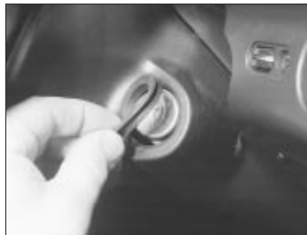
28.4B . . . remove the rubber ring . . .
