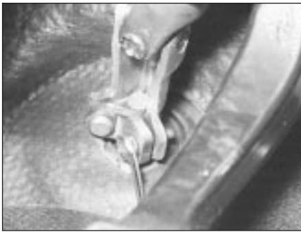
28.6A Unscrew the clamp plate bolt . . .
