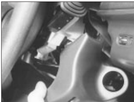
28.4C . . . and remove the lower shroud
