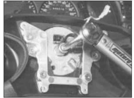
27.9 Tightening the steering wheel retaining bolt
