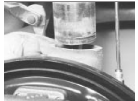
11.11 Separating the knuckle from the strut
