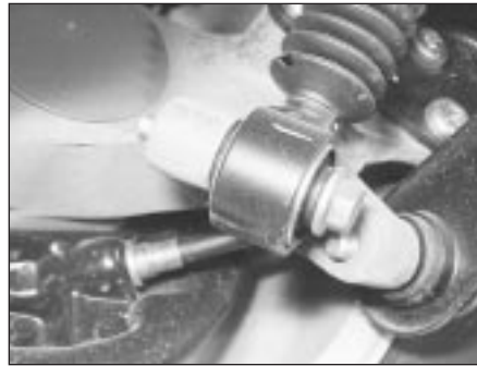
19.3 Rear shock absorber lower mounting bolt (Estate)
