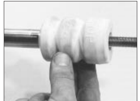
5.5D Removing the bump stop
