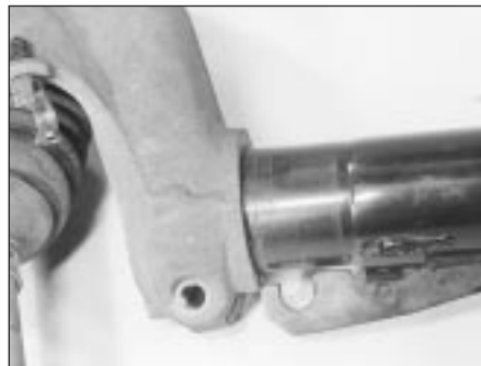
4.12B Releasing the knuckle from the strut
