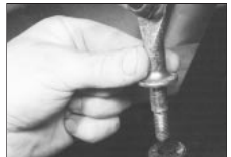
13.2C . . . and remove the anti-roll bar link from the lower arm
