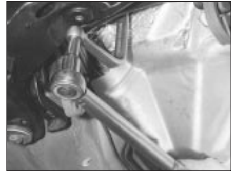
30.9 Tightening the steering gear mounting bolts using the U-shaped spanner (arrowed)
