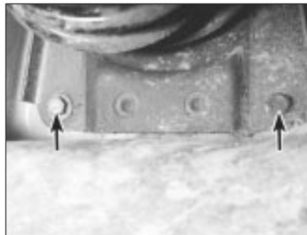
11.13 Bolts (arrowed) securing the strut upper mounting to the underbody
