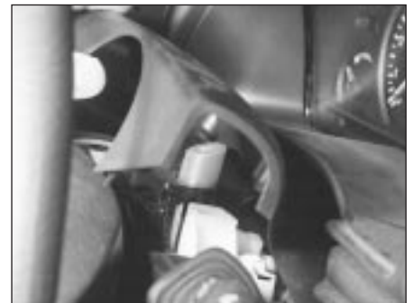
28.4E Removing the upper shroud
