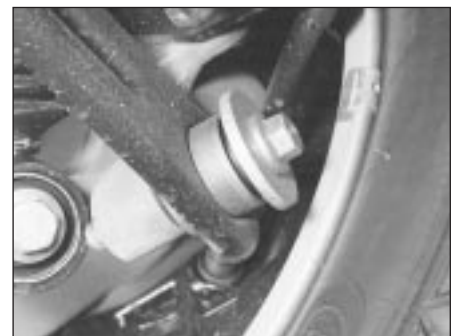
21.6 Front lower arm-to-knuckle mounting bolt
