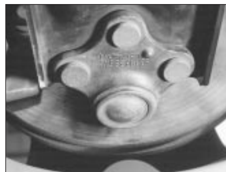
8.0 Original riveted front suspension lower arm balljoint
