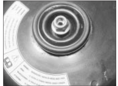
4.10 Front suspension strut upper mounting nut
