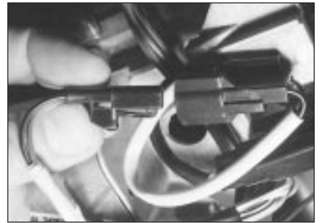
28.7B Disconnecting the small multi-plug . . .
