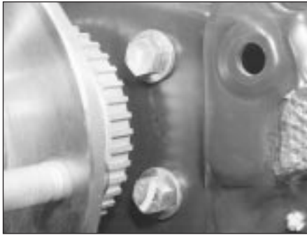
10.5 Two of the bolts securing the brake backplate to the rear suspension knuckle
