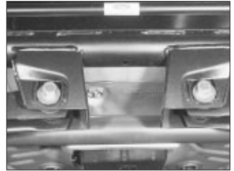
22.3 Bolts securing the rear lower arms to the crossmember - note the eccentric spacers
