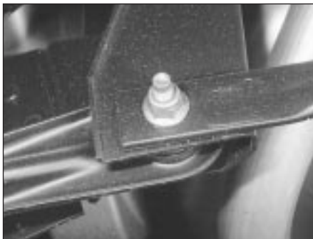
23.2 Front lower arm-to-crossmember securing bolt
