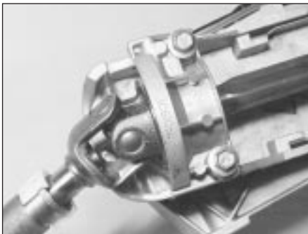
28.9 Steering column and universal joint
