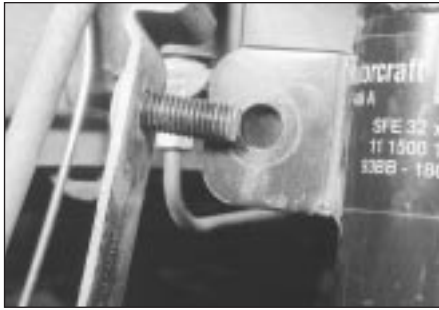
4.2 Removing the brake hose support bracket from the front of the front suspension strut
