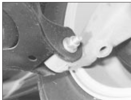
21.5 Rear lower arm-to-knuckle mounting bolt
