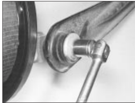
11.9A Unscrew the bolt . . .
