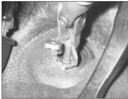
28.6B . . . and swivel the clamp plate around
