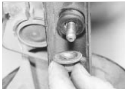
13.2B . . . remove the nut and rubber bush . . .
