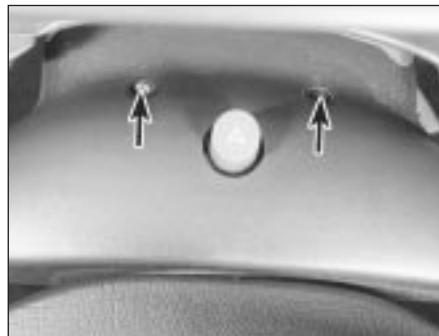
28.4D Upper shroud retaining screws (arrowed)
