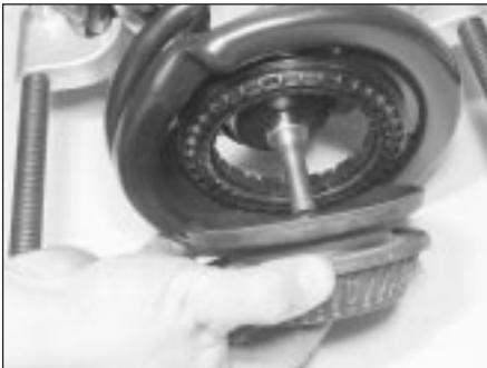
5.5B Removing the top mounting from the strut
